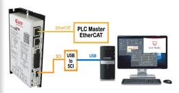
IDE e3PLC configuration (programmable) - c0690
