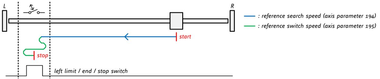
Figure 4.5: Search left stop switch from both sides
