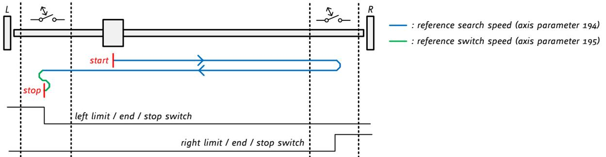
Figure 4.3: Search right stop switch, then search left stop switch
