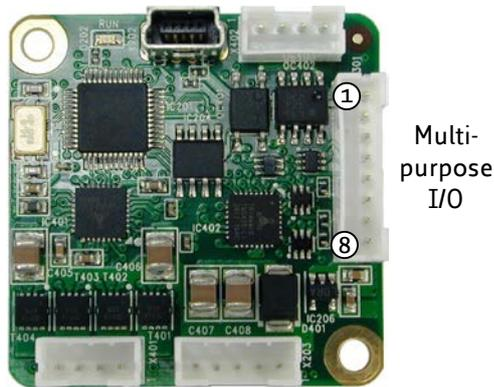
Figure 3.2 I/O connector
