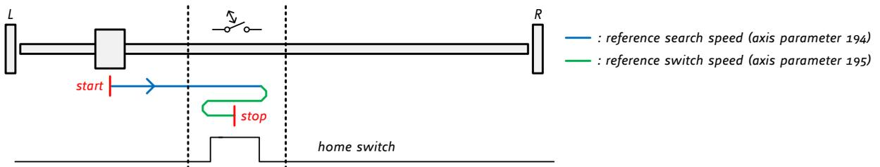
**Figure 4.9: Search home switch in positive direction, ignore end switches**
