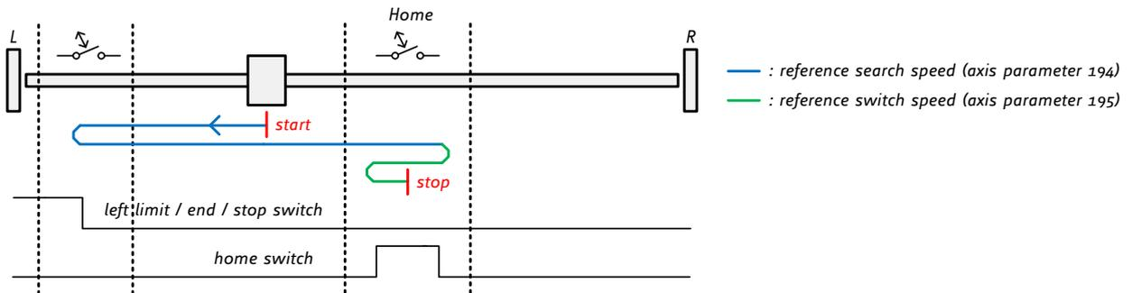
Figure 4.6: Search home switch in negative direction, reverse direction in case left stop switch is hit
