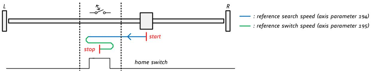
**Figure 4.8: Search home switch in negative direction, ignore end switches**
