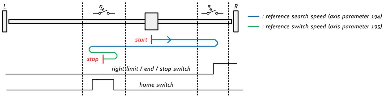
**Figure 4.7: Search home switch in positive direction, reverse direction in case right stop switch is hit**
