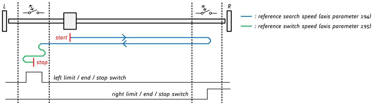
Figure 4.4: Search right stop switch, then search left stop switch from both sides
